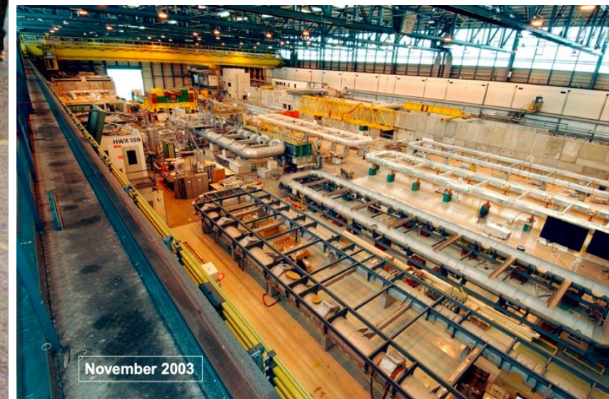
Barrel Toroid coil integration and testing in Hall 180 (CERN)
