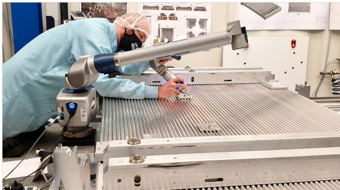
sMDT chamber measurement (MPI)
