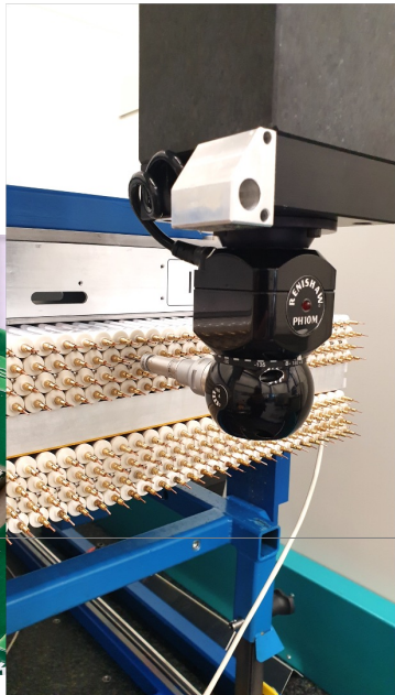
sMDT geometry measurement (MPI)
