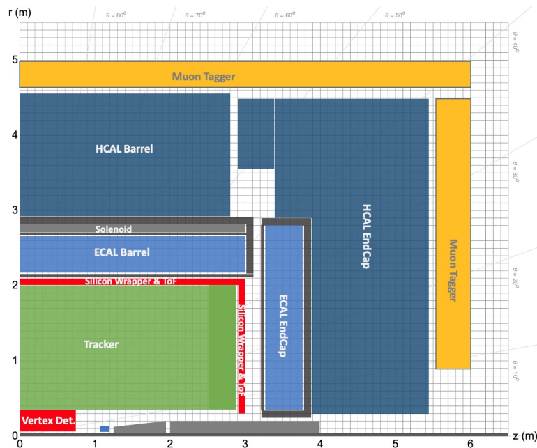
ALLEGRO detector concept around noble-liquid EM calorimeter [Ref]
