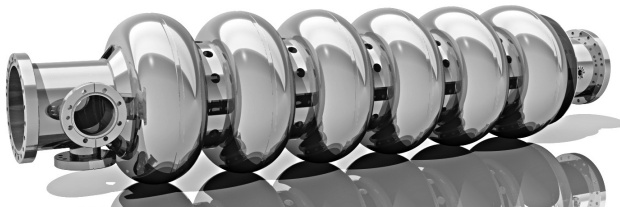
Compact 800 MHz cavity (~20 MV/m), 6-cell, bulk Nb, Nb 3 Sn if R&D is successful
