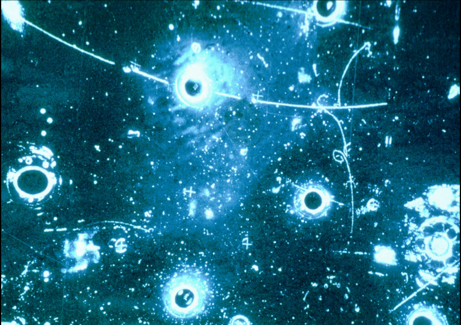
Event shows tracks produced in the 1200 litre Gargamelle bubble chamber that provided the first confirmation of a neutral current interaction (image: CERN)
