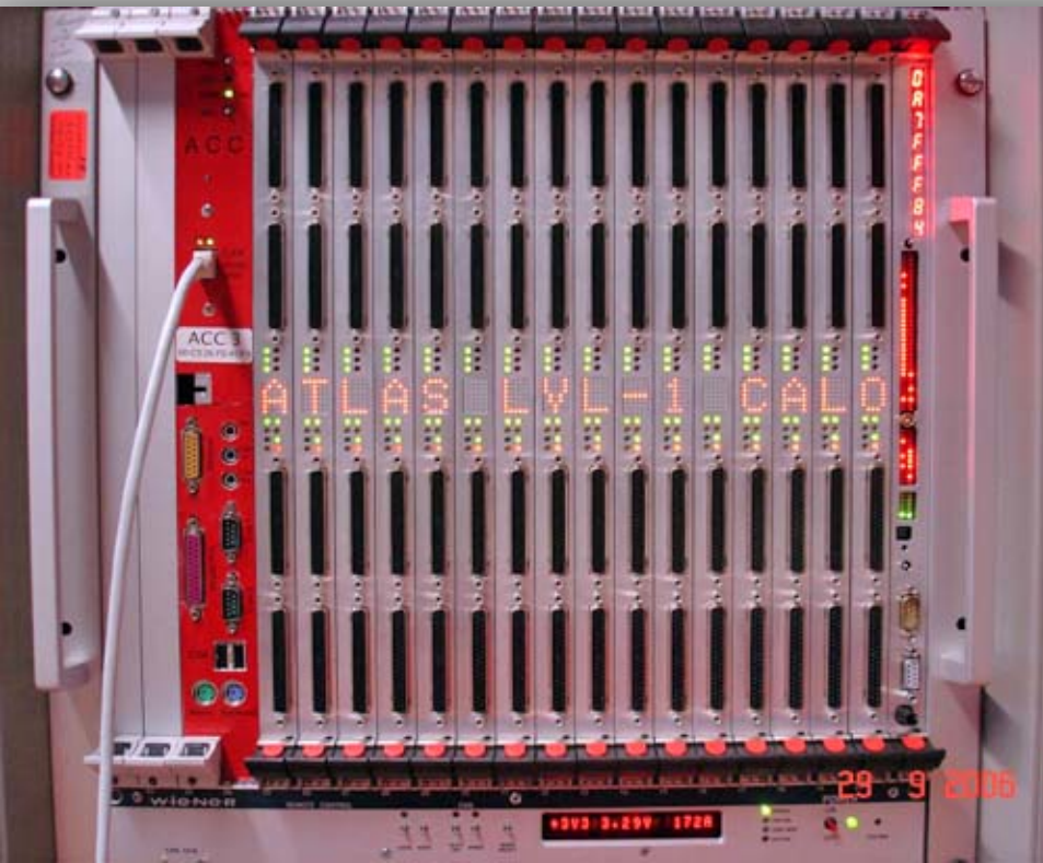
Level-1 Calorimeter Pre-processor crate
